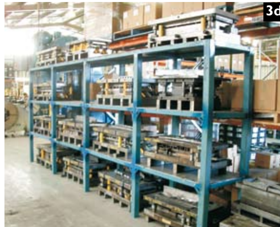
Waste not, want not: OzPress goes through a lean overhaul, using 5s as one of its start off points. The company optimised its layout and product-flow to reduce downtime. 3a) without flow racks 3b) with flow racks 3c) without tool racks 3d) with tool racks
