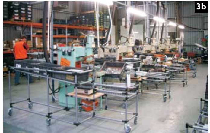
Waste not, want not: OzPress goes through a lean overhaul, using 5s as one of its start off points. The company optimised its layout and product-flow to reduce downtime. 3a) without flow racks 3b) with flow racks 3c) without tool racks 3d) with tool racks
