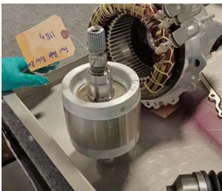
"Secret weapon": Tesla opted for an aluminum rotor in its front induction motor on the Model Y, as opposed to copper in the Model 3.
